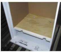
Board-type heat insulating material
