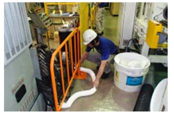
Flow prevention drill simulating the leakage of oil. Nihon Plastic Co., Ltd. (Headquarters factory)
