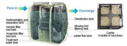
Perspective diagram of compact wastewater treatment unit KZ-type and high-performance carrier
