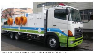
Drainage Pump with Vehicle for Disaster Recovery
